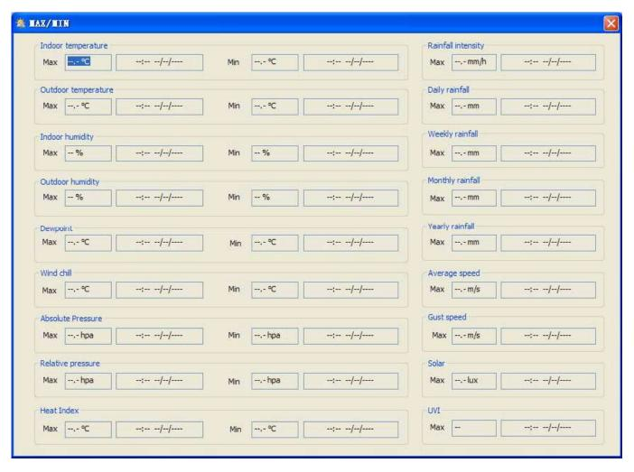
This section is used to display the recorded min and max value recorded with time stamp.
